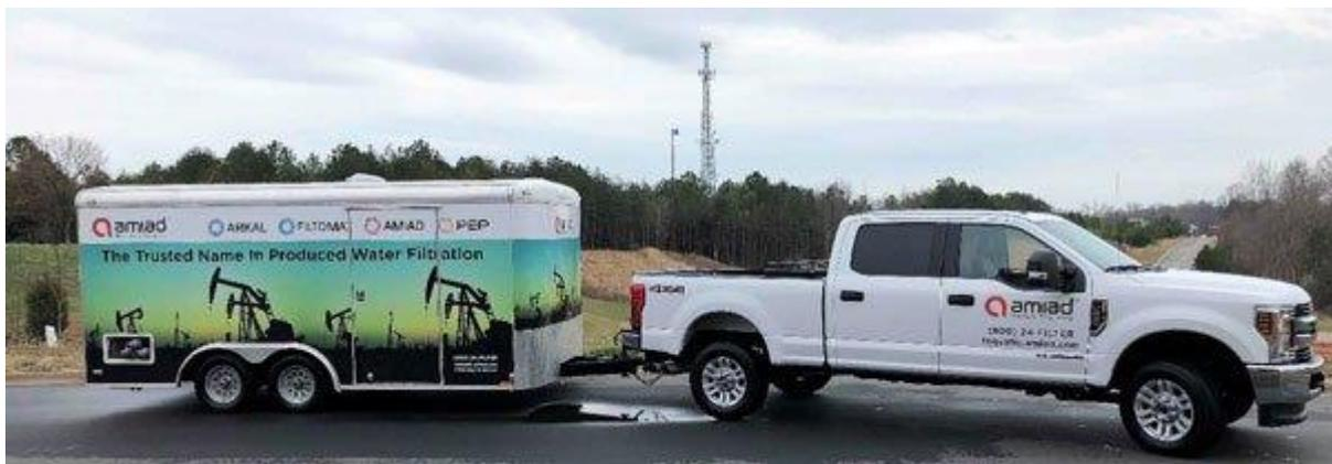
The TEQUATIC™ PLUS Oil and Gas Demo Trailer is a mobile self-contained and fully operational unit equipped with a state-of-the-art F75 TEQUATIC™ PLUS filtration skid configured to run as a pilot unit for produced water applications in oil fields across the country.
