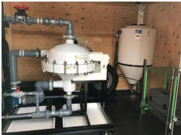
The system only requires an external power source and includes a complete filtration skid, a feed pump, and a concentrated solids collection system.
